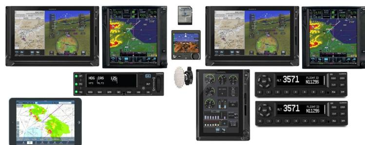
Touchscreen \* ADS-B in and out \* WAAS equipped \* Traffic Screen On-Board Radar & Nexrad Weather \* Terrain \* Approach Plates \* STARS/SIDS \* Visual Approaches \* VNAV \* Synthetic Vision \* Victor Airways \* Moving Map Waypoint Info \* HSI Mapping \* SiriusXM Satellite \* SafeTaxi Charts .\* Standby Instruments Apple IPAD for ForeFlight or Garmin Pilot with Bluetooth to ADS-B
